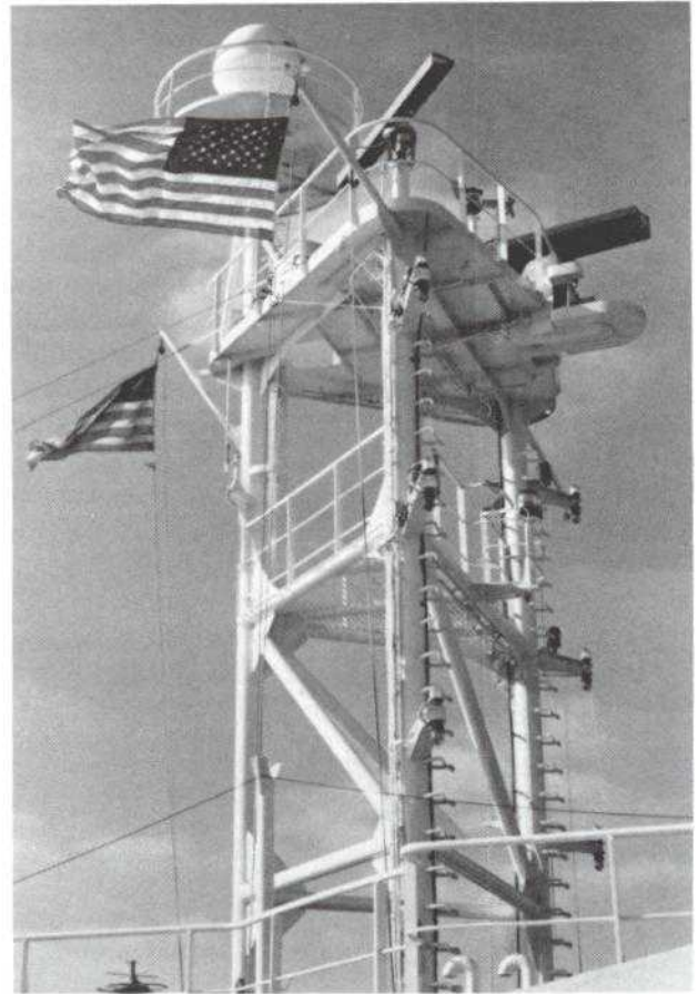
Figure 7. MCS-9100 shipboard antenna terminal
