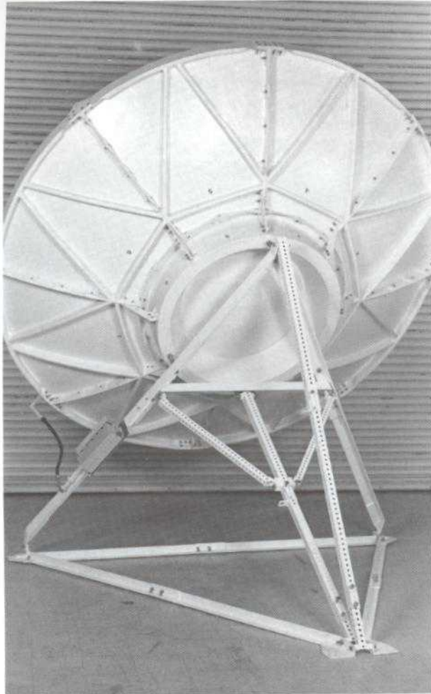
Figure 21. 2.9-m transportable antenna system (rear view)
