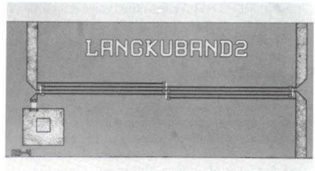
Figure 12. Lange coupler on a 50-mm-diameter GaAs wafer delivered to Hughes Aircraft Company
