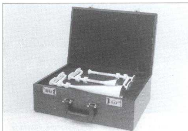
Figure 12. 35-GHz horn gain standard built by MTSD and used by NIST
