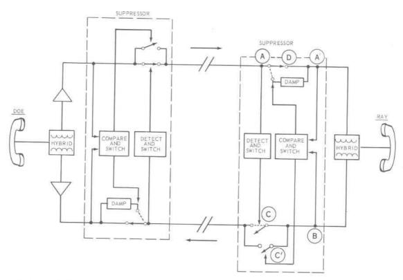
Figure 1. Long-distance telephone circuit with echo suppressors. When either party is talking alone, the suppressor at the opposite end opens the return path so no echo can be transmitted.
