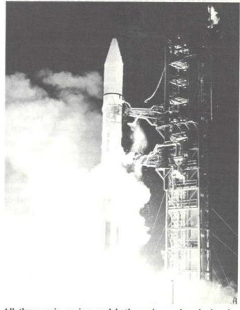
All three main engines and both vernier engines ignite simultaneously as the Atlas-Centaur, which will carry the IN-TELSAT IV into synchronous orbit, lifts off the launch pad under the combined booster-sustainer-vernier-engine thrust
