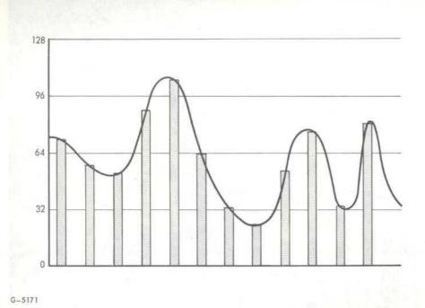
Analog voice wave is sampled and quantized into 128 levels.
