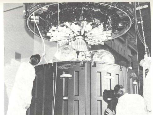
Engineers at Hughes Jet Propulsion Laboratory in Pasadena, Calif., check the fit of the solar cell casing on the INTELSAT IV satellite now in production. Launching of the Series IV satellite is scheduled by INTELSAT for mid-1971.
