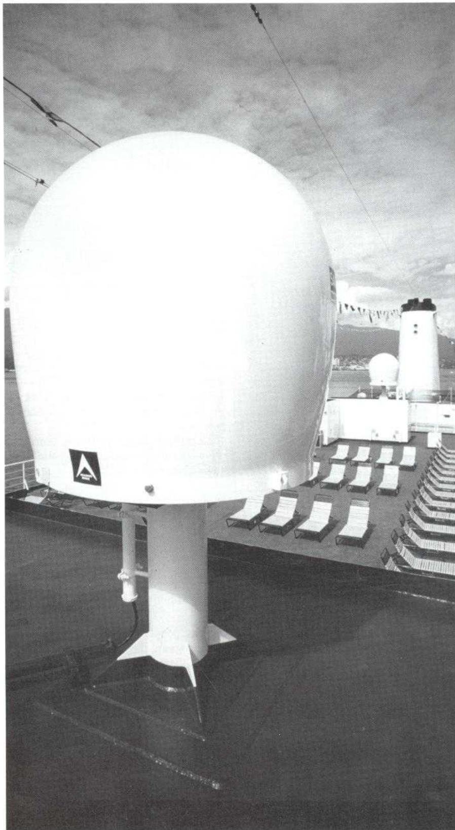
**A close up of the latest in satellite communications technology for cruise ships... the ship earth station (SES).**
